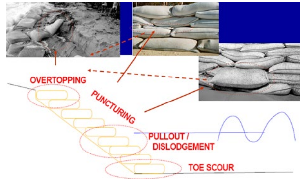
Figure 2 Examples of the four typical failure modes for SFGC walls. (Source: [22])
