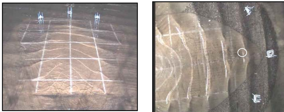
Figure 4: Extracted images from oblique and overhead video showing wave transformation suitable for surfing over the reef.
